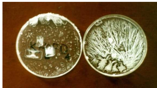
Fig. 3. \text{KH}_2\text{PO}_4 crystals. Left: the evaporation of solutions from the anode department of the electrolyzer formed crystals of the cubic form; right: the evaporation of solutions from the cathode department – the needle-shaped crystals.
