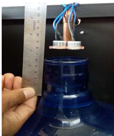
Figure 9. Water level measurement with sensors.
