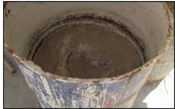
Figure 4. Non-usable lime owing to the cracked lime after losing all water content.
