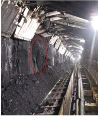
Figure 1. Photo of rib spalling.
