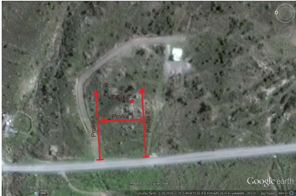
Figure 4. The location of MASW measurements realized in GNSS station; DEU5 and its surrounding. (Red arrows represent the MASW profiles and their directions.)
