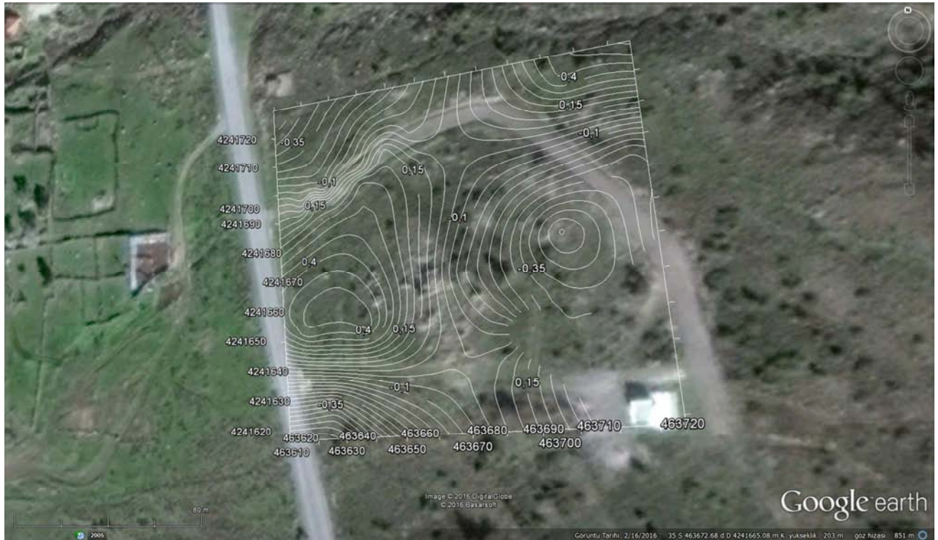
Figure 8. The Bouguer gravity anomalies obtained by applying terrain corrections and removing the 2 nd trend for DEU5 and its surroundings.
