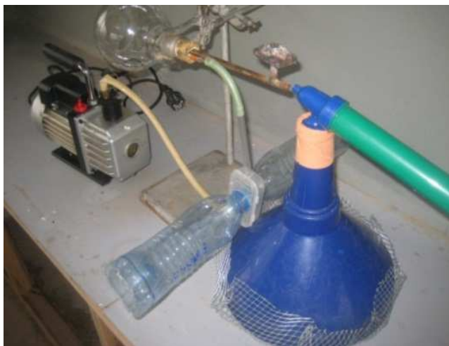
Figure A1. Nose-only Smoke Inhalation Apparatus.
