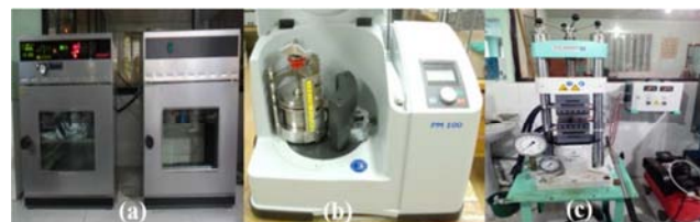
Figure 1. Photographic image of the instrumental set-up (a) Vacuum oven (b) planetary ball mill (c) W/P hydraulic press machine.
