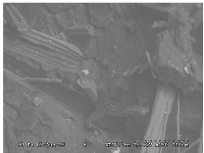
Figure 8. SEM of fracture surface of 10% untreated PPJC.
