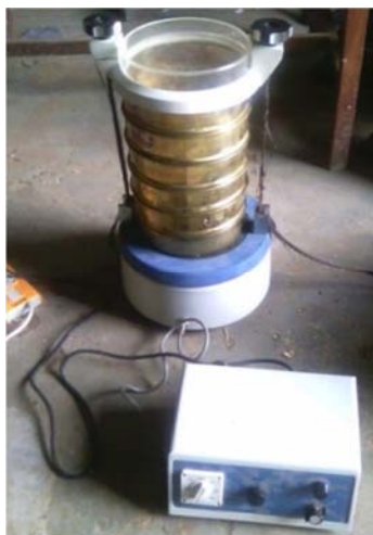
Figure 1. Fritsch shaker machine with sieve stack mounted and amplitude box.
