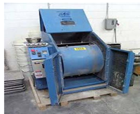
Figure 3. LOS Angeles Abrasion Test on Aggregates.
