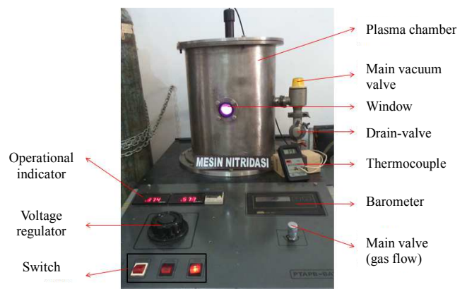
Figure 2. A DC-plasma glow discharge in PSTA-BATAN Yogyakarta.
