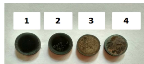
Figure 6. The samples after nitridation with various % of Argon. Labels 1, 2, 3, and 4 indicate the percentages of Ar; 10%, 20%, 30%, and 40%, respectively.
