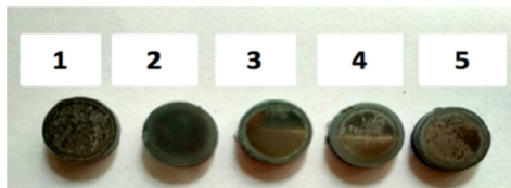
Figure 3. The samples after nitridation and Argon post-treatment. Labels 1, 2, 3, 4, and 5 indicate the post-processing times; 10, 20, 30, 40, and 50 minutes, respectively.
