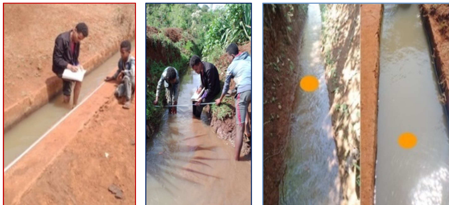
Figure 2. Discharge measurement by area-velocity method.
