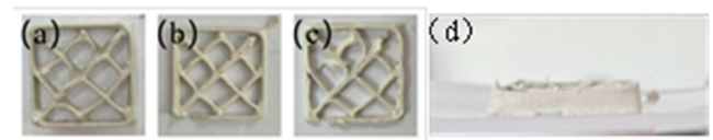
Figure 4. DSW printing results of 0% (a), 5% (b), 10% (c), and 15% (d) (w/w) PEG content while maintaining the TiO 2 :H 2 O ratio at 3.5.
