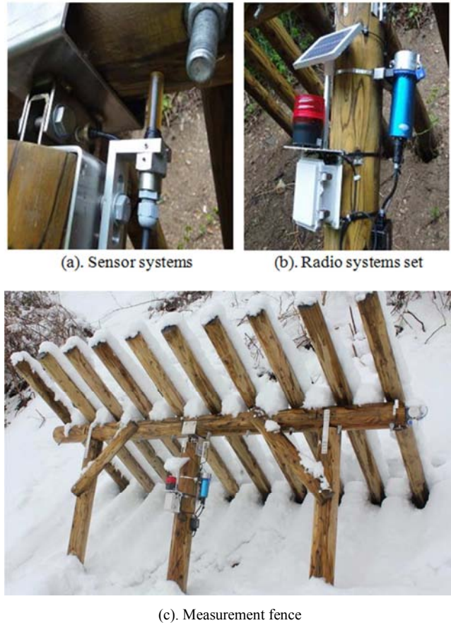
Figure 1. Avalanche fence for peril measurements.
