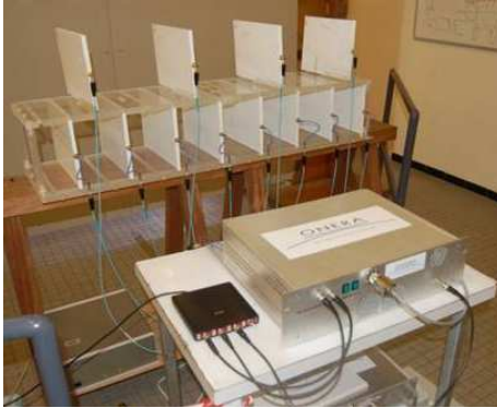
Figure 6. Picture of the realised time multiplexed ultrawide band MIMO radar.
