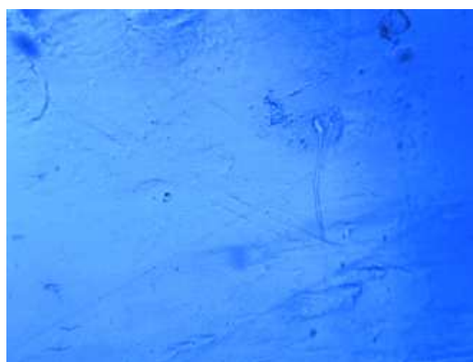
Fig. 6. Etch patterns observed of HA Single Crystal
