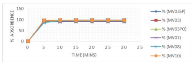
Figure 13. Effect of contact time on methyl blue adsorption onto Metal Oxide composite.
