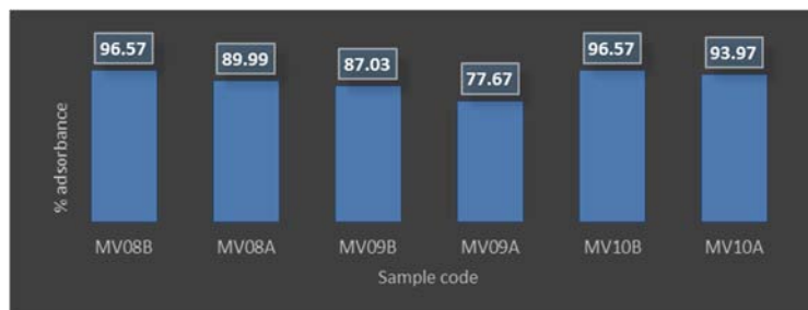
Figure 10. % absorbance before and after adsorption, for Clay based composites.
