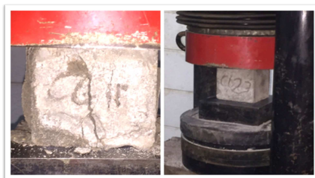
Figure 1. The concrete pattern where ever measuring its resistance by the presses.
