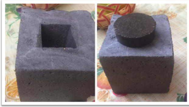
Figure 2. Form of the template in which the dose measurements were done.
