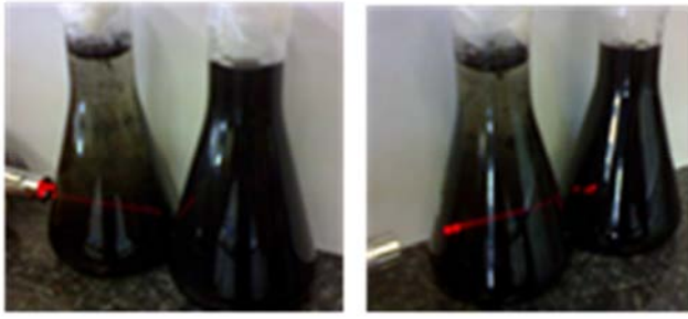
Fig. 2. Comparison of the stability of the SDS stabilized CNTs suspension (the right one) with the unstable CNTs suspension without SDS (the left one). The photos were taken after 3 days pH of both suspensions was kept 10.
