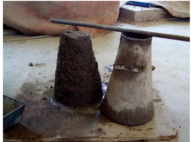
Figure 2. Measurement of workability of concrete.
