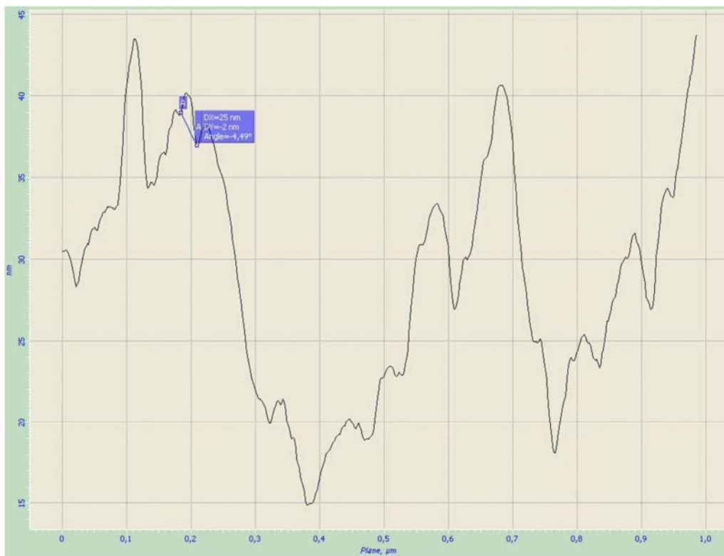
Figure 2. Surface relief of the Pb-VCT sample with vacancy cluster tubes images. The characteristic surface scales are determined using a power spectrum (Fourier analysis), Femtoscan online software applied.
