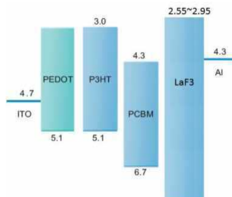
Figure 2. Energy diagram with \text{LaF}_3 buffer layer [13].
