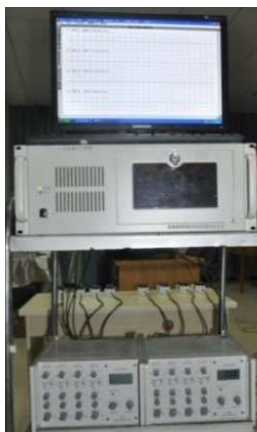
Figure 3. Ultra-dynamic strain testing system.
