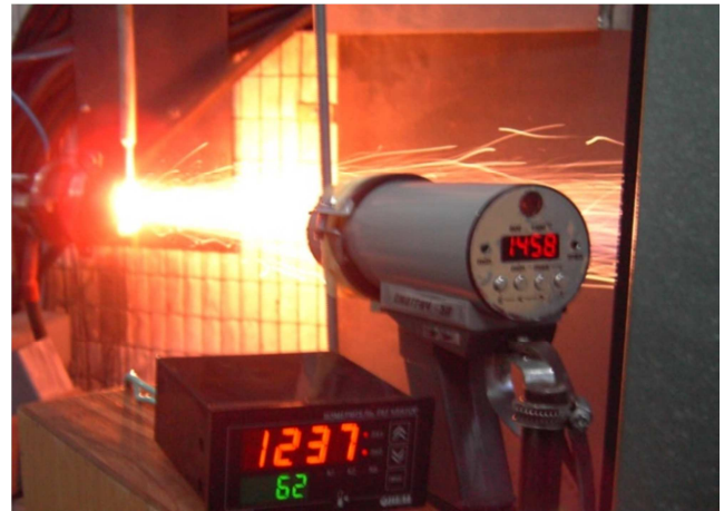
Figure 4. Plasmatron with CWF ignition in operation.
