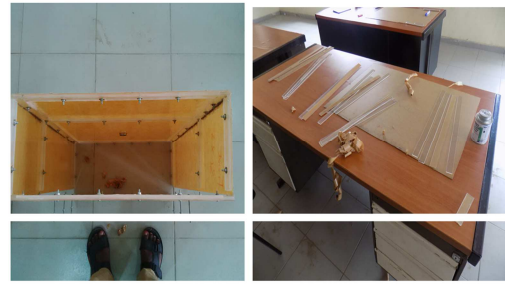
Figure 6. Construction of the turbine casing according to the designed dimensions.
