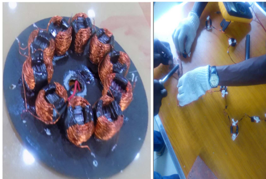
Figure 9. Terminated ten (10) Coils Stator Windings and soldering of its joints.
