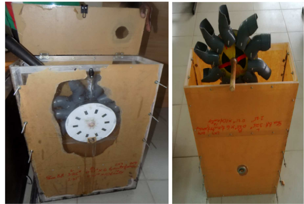
Figure 10. Constructed and Assembled Turbine System.
