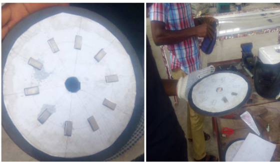
Figure 8. Construction of Rotor part of the Alternator.
