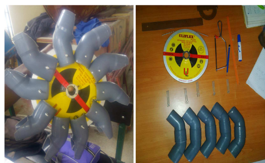
Figure 7. Some Materials Used for Turbine Component and the Constructed Turbine Blade.
