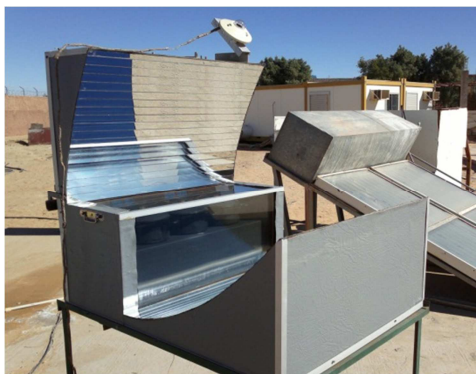
Fig. 2. The stationary box-type solar cooker equipped with an asymmetric CPC.
