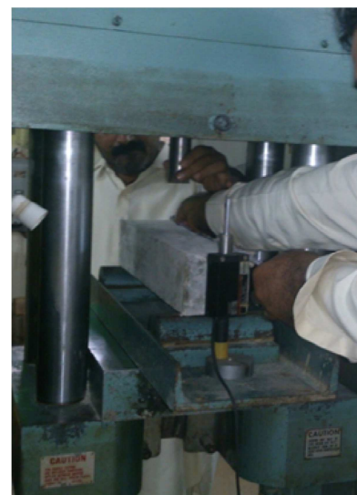
Figure 3. Shows Testing Strength Flexural Specimen in UTM.
