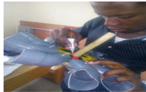
Figure 10. Fixing of shaft to the turbine wheel.
