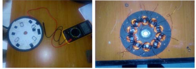
Figure 4. Stator coil (testing and construction).
