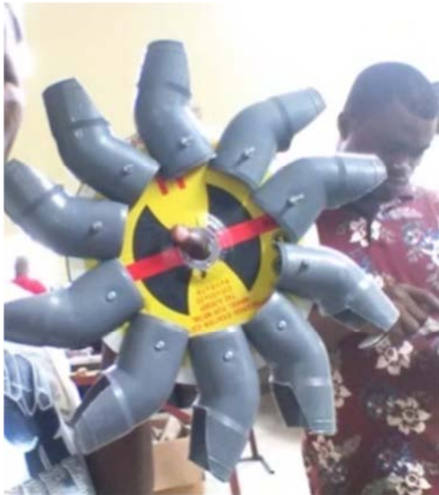
Figure 3. Pelton turbine wheel (FRONT).
