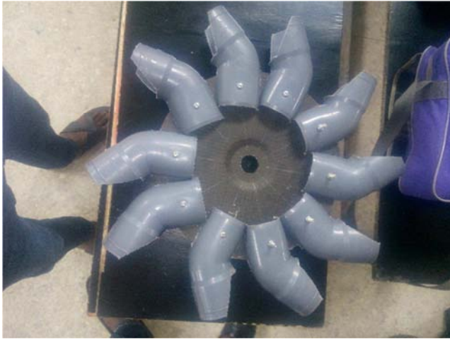
Figure 2 Pelton turbine wheel (BACK).
