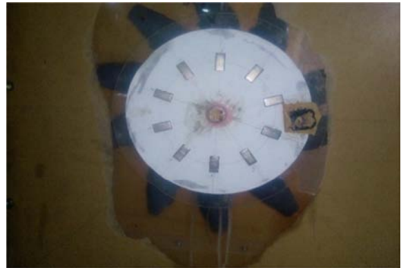
Figure 5. Rotor (N50 Neodymium magnet).
