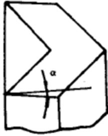
Fig. 2. Cross-sectional view of V-shaped seal ring.
