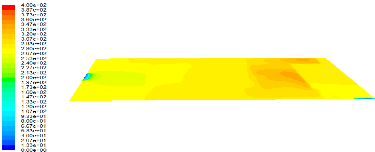
Figure 3. Contours of radon concentration ( \text{Bq m}^{-3} ) in closed Hammam at plane ( Y=1.50 \text{ m} ).
