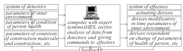
Figure 4. Scheme of functioning of intellectual building
