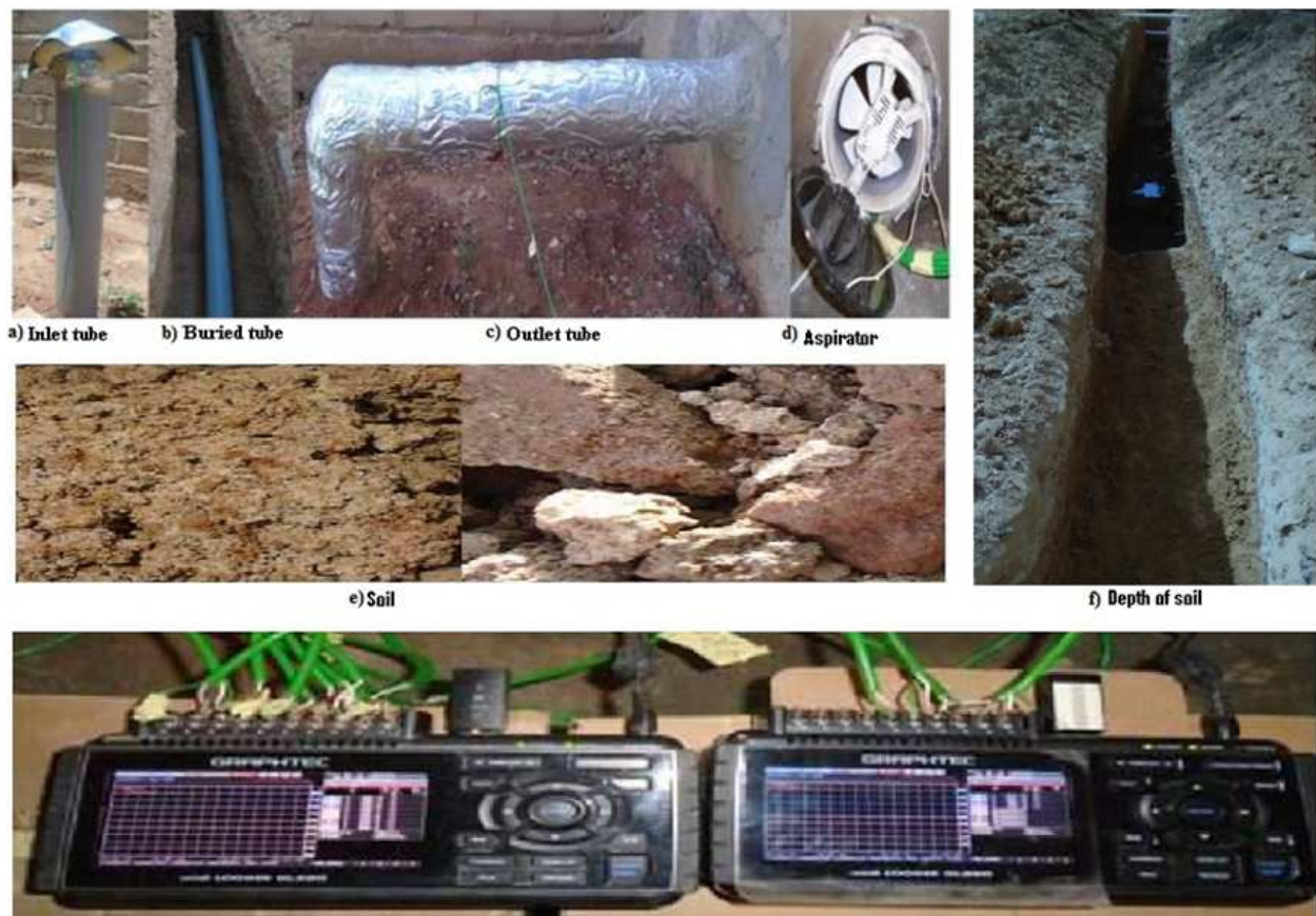
Figure 2. Description of some parts of experimental device.
