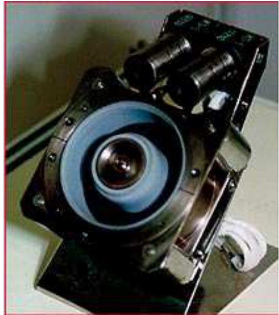
Figure 4. Electrojet engine SPD-100 [6].
