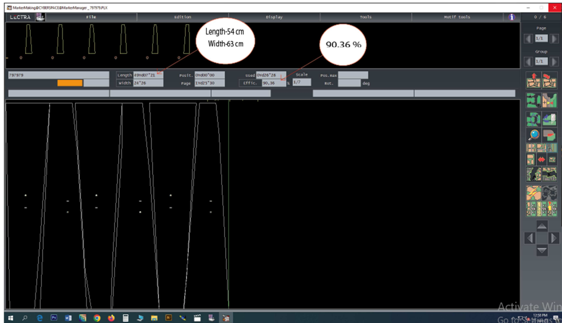
Figure 8. Zero waste gored skirt pattern.
