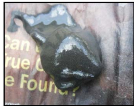
Figure 13. Wax model coated with charcoal-clay mixture.
