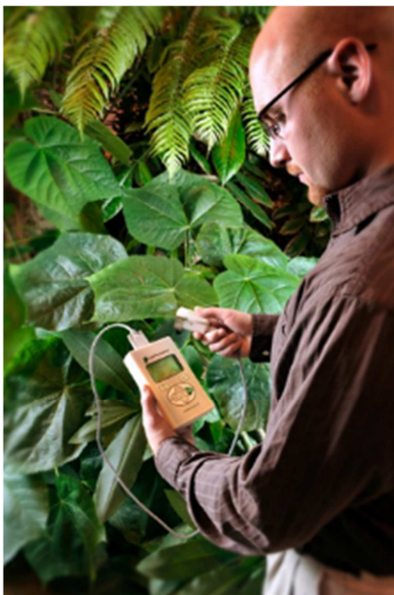
Figure 3. Steady state porometer measuring stomatal conductance.
