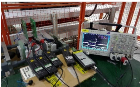
Figure 4. Equipment of series-connected IGBTs.
