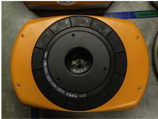
Figure 2. Kiva robots are equipped with cameras.
