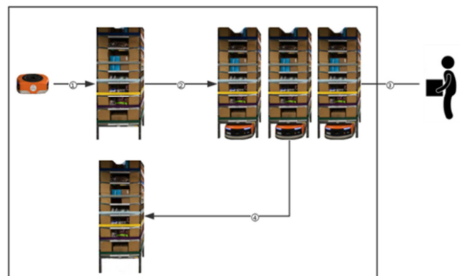
Figure 3. Four steps of Kiva robot complete the order task.
