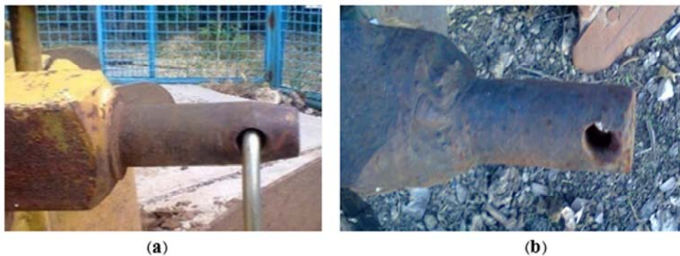
Figure 11. The left pin of crossbar; a) healthy pin and b) broken and welded pin.
